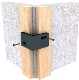
**2** - Place the corner finishing profile on the brackets and drill through the profile, the purpose of this operation being to mark the brackets underneath.
