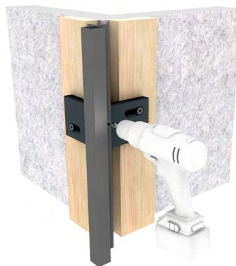
**3** - Drill the brackets with a drill bit slightly smaller than the diameter of the assembly screws to ensure that the screw anchors securely into the bracket.
