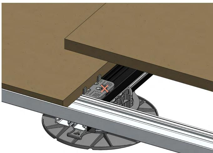
If necessary, the tabs on the slab support can be broken off with pliers.
