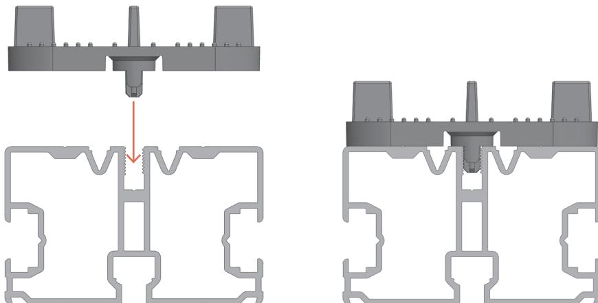
Position the slab support in the central groove of the rail; it is not necessary to screw the slab supports in place.
